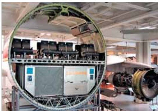
Airbus A300 fuselage cross-section, showing the passenger compartment above and LD-3 cargo containers below. On display at the Deutsches Museum in Munich, Germany (Asiir/Wikipedia)
