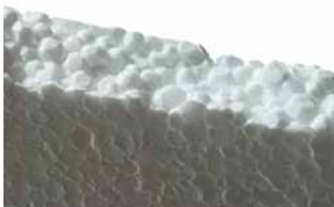
Expandable polystyrene beads (XXL Photo, Shutterstock)
