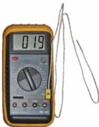
Thermocouple connected to a multimeter displaying room temperature (Sovxx, Wikipedia)
