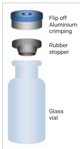
A primary container closure system with flip off, aluminum crimping and rubber stopper (Kartoglu)
