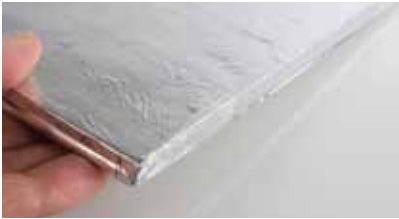
A vacuum insulation panel (diepre, Shutterstock)
